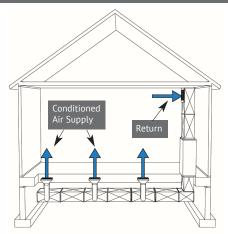
By locating the air handler and the return ducts in the main part of the house, the air exchange between the crawl space and the house is minimized.
