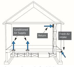
As one compliance option for whole-house fresh-air ventilation, a controlled amount of fresh air is supplied to the air handler return located in the closed crawl space.
